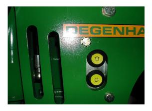
Mount the plate included in delivery at the side plate of the front hitch with the switches.
