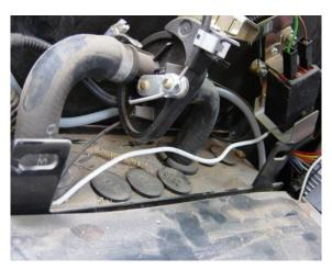
Install the cable at the side next to heating hoses to the rear.
