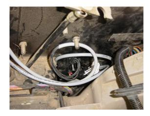
Put the control box at the side next to the air duct and the temperature governor in the cavity.
