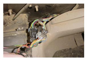
Separate cable harness of electric joystick at the 6- and 8-pole plug.
