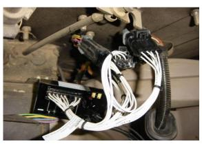
Interconnect the adapter cable included in delivery and connect the remote control module at the designated compact plug. Also insert the feeler cable harness in the module.
