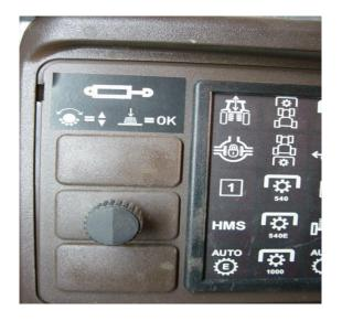
Connect all plugs according to the instructions in the tractor and take the feeler cable harness with you into the cabin. Choose the respective control unit by means of the selector switch for the hydraulic valves and select lifting or lowering to prevent display from changing after a short while.
