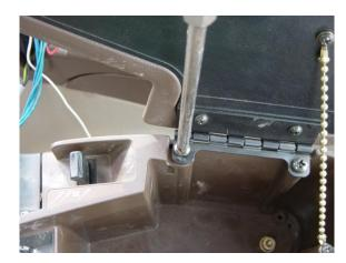
Remove the three lower bolts at the Command-Armrest and dismount crosshead screw of the cover at front. Now the upper operating unit of the armrest can be lifted upwards.
