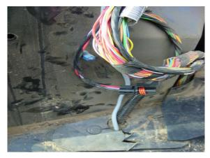
Remove multi-standard socket from the outside at mud guard by means of two bolts. Lift floor rubber mat and remove fixing nuts at the side console.
