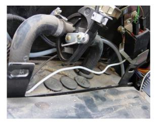
Cable to be installed at sides next to the heating hoses to the rear.
