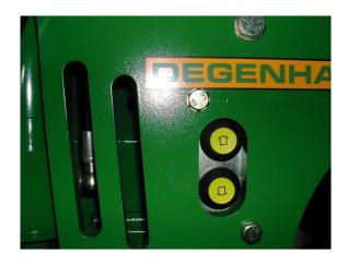
The plate as included in deliver at the side plate of front hitch to be mounted with switches.
