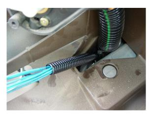
Push the cable harness for remote control through the lower half of the armrest an connect it to the original cable harness by use of cable retainer.
