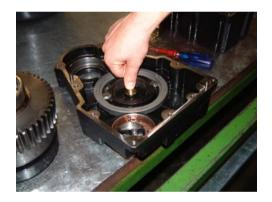
Check condition of the bronze mechanical seal, replace if necessary, replace the o-ring on the bronze mechanical seal. Replace all oil seals.
