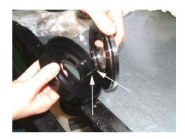
Remove the piston from the cylinder. Check sealing surfaces and dowel pins for damage.
