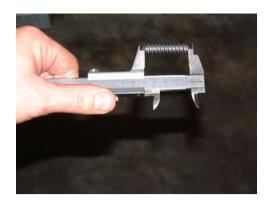
Check the length of the compression springs from the clutch, length = 42.4 mm
