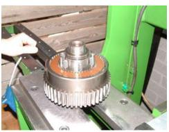
Check if the dowel pins are free and not damaged.
