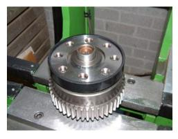
Check the surface where the bronze mechanical seal contacts the clutch unit. If the surface is damaged the shaft will have to be replaced.
