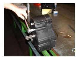
Remove all the 10 M8 Allen bolts bolts, which are located around the PTO unit. The 2 bottom centre bolts are mounted with a dowty-seal washer. Oil can be drained from these points also.
