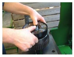
The complete cylinder can now be removed from the clutch unit.
