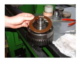
Replace the clutch plates if worn or damaged. Place the paper and metal plates alternate in the clutch. Start and end with a paper plate.
