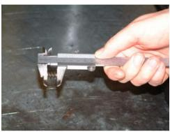
Check the length of the spring from the mechanical seal length = 13mm.
