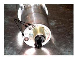
Take care: Do not leave the seal rings in the PTO unit after removal of the pump.
