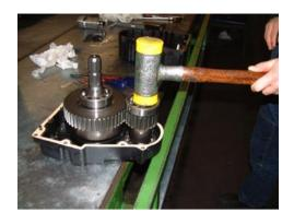
Place the clutch and the pinion in the rear half of the PTO unit.
