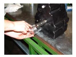
Assemble the pump in the PTO unit with the two M6 bolts taking care with the o-rings. Fill PTO with oil to the level plughole. If PTO was fitted with an oil cooler remount onto tractor, refit cooler then fill with oil too oil level plughole. After mounting, run PTO then recheck oil level and adjust as necessary.
