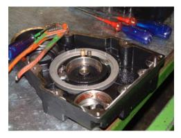
Dismantle the mechanical-seal (Bronze bush). Do a visual check of the working surface of the bronze bush.
