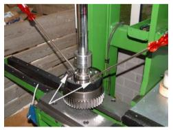
Carefully lever bearing off rear of clutch unit.
