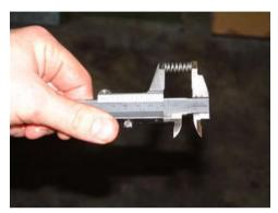
Check the length of the compression springs from the dowel pins length = 22.5mm.
