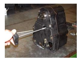
Remove the sensor by removing the M5 bolt; also remove sensor o-ring seal.
