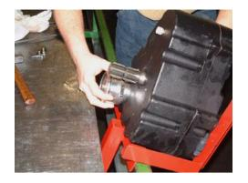
Pull the pump out of the PTO unit from the front.
