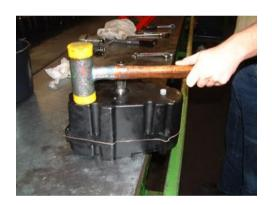
Use a rubber/plastic hammer to assemble the PTO.
