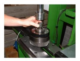
Clamp the clutch unit using a press.
