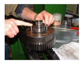
Replace the dowel pins with the springs. Important! The round side must be pointing upwards.
