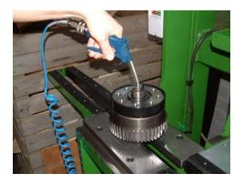
Check the clutch for correct operation using air pressure as shown.
