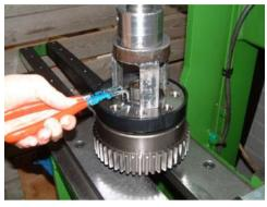
Using a press apply light pressure to the clutch piston and remove the circlip.
