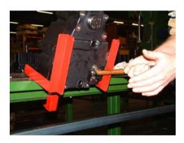
When the 2 M6 bolts are removed, the pump can be taken out of the PTO unit (from the front). Gently tap or apply pressure to rear of the pump unit.
