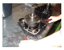
Pull the complete clutch unit out of the PTO, use 2 screwdrivers to lever up the clutch unit from the rear half.
