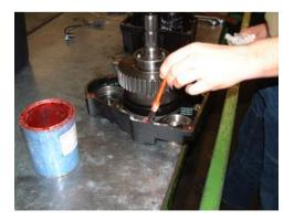
Grease the gasket surface so the gasket remains in place during assembly.
