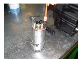
Before mounting the pump, replace all the o-rings; assemble the small o-rings at the rear of the pump with grease.
