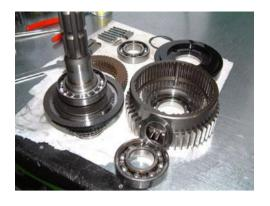
Clean and examine all the parts for wear or damage. Check all the sealing surfaces for damage. Replace all seals.
