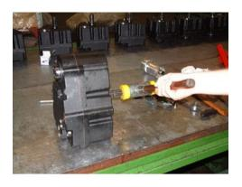
Hit the output shaft with a rubber or plastic hammer in axial direction, to separate the 2 sides.
