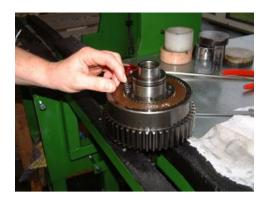
Place the compression springs back in the clutch.
