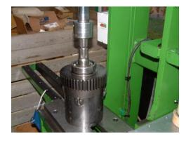
Press the output shaft out of the unit.
