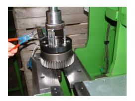
Slide the cylinder with the piston onto the shaft, apply pressure to piston then fit the circlip.
