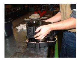
Place the front PTO unit half over the shafts.
