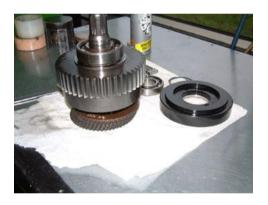
With the output shaft facing upwards tip the clutch plates out of the clutch housing.
