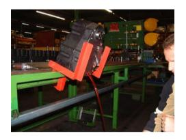
After removing PTO unit from tractor, remove drain plug from rear of PTO and drain the oil. If PTO was fitted with an oil cooler the cooler return pipe connects at the drain plug port therefore oil will be drained before removal of PTO unit from tractor.
