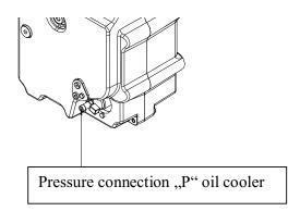
Tighten the screw-nipple to the gearing of the front PTO.
