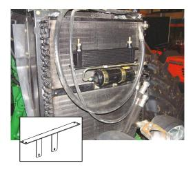
Mount the retainer of the oil cooler together with the dryer of the air conditioner in front of the JD-radiator package.
