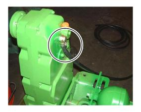
Mount the runback hose of the oil cooler to the PTO gear.
