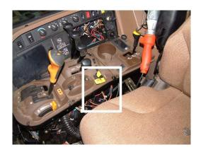
Mount PTO switch at a suitable place. Connect cable harness for the switching of PTO according to the wire diagram on the following pages.
