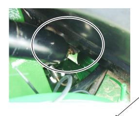
Mount the supplied hydraulic hose in between the membrane-accumulator at the front PTO and the original connection (rotating joint).
