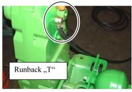
Pass the runback hose of oil cooler and connect it to the oil cooler. Fix hose with hose clamps. Make sure, that there is abrasion at the cable harness.
