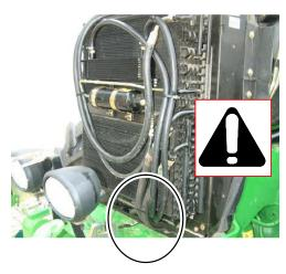
Insert and connect oil cooler hoses according to the picture.
