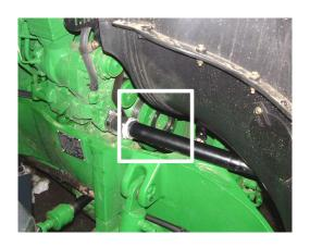
Remove the paint on the contact area of the v-belt pulley.
