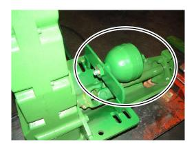
Mount the membrane-accumulator at the provided mounting of the front PTO.
