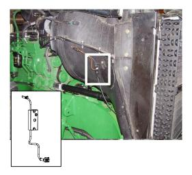
The Switch-on deceleration relay can be mounted to the radiator protection on the right side of the tractor by using two bolts M5 x 30 and nuts. Put the cable harness to the magnet valve of the PTO and connect it.
