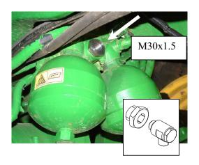
Mount the supplied thread-reducing fitting (arrow) (M30x1,5) at the position of the air vessel with membrane. Reuse the old joint ring of the accumulator. Fasten the screw (rotating joint).
